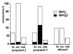
products ratio through the dehydrogenation and dehydration as well as the effect on these parameters of pre-treatment conditions of ND and of alcohol nature (see, for example, the Figure at 330°C).
