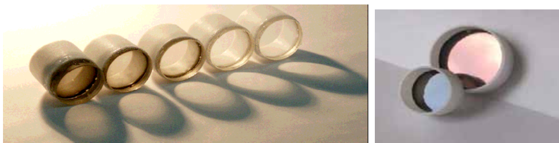
Fig. 1. The mirrors and filters covered with polymer films containing individual SWNTs.
