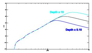
Since plasma is more optically thin to higher frequencies, any change in viewing depth affects their intensities more than for lower frequencies. The optically thick nature of plasma with regards to lower frequencies means that a change in depth of plasma has an only negligible effect on the amount of radiation emitted, as the radiation emanating from deeper layers is absorbed regardless of the depth of measurement.
