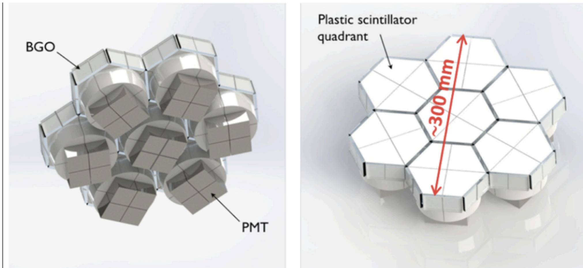
**Figure 1:** Overview of the SPHiNX detector. Avalanche photodiodes for reading out the BGO scintillators are not shown.
