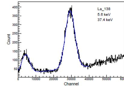
re 5. The spectra of <sup>55</sup>Fe and <sup>138</sup>La radioactive sources. The energy resolutions are 95.6% at 5.9 keV, 126.6% at 5.6 keV and 24.1% at 37.4 keV.
