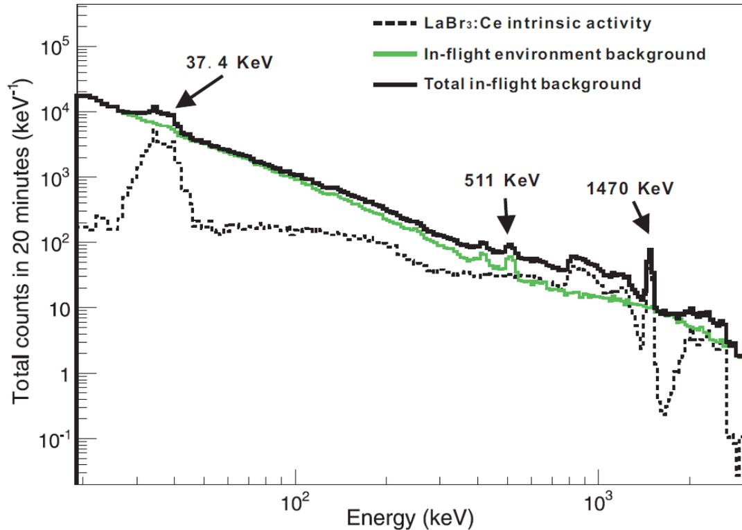
Characteristic lines for in-flight gain calibration
