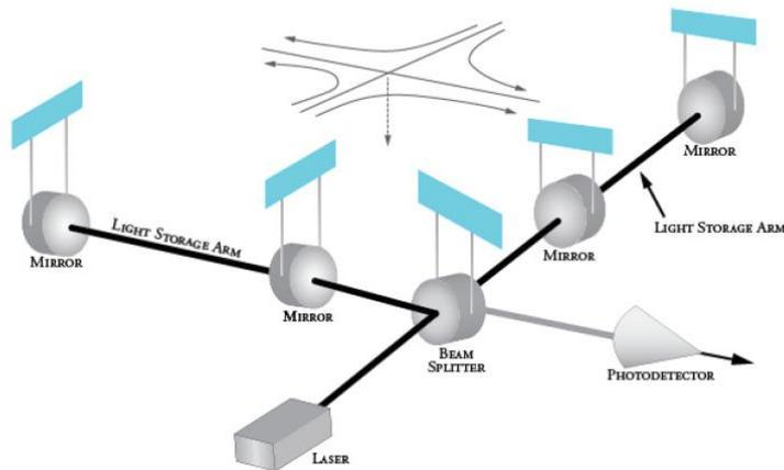
**FIGURE 4.** Schematic drawing of a ground-based laser interferometer for GW detection. The beam splitter sends light down the two arms; the beams are then interfered at the photodetector. A passing GW changes the arm lengths, causing phase changes in the laser beams. These phase changes appear in the interference patterns at the photo detector, giving the GW signal. Figure courtesy of the LIGO Laboratory, used with permission.
