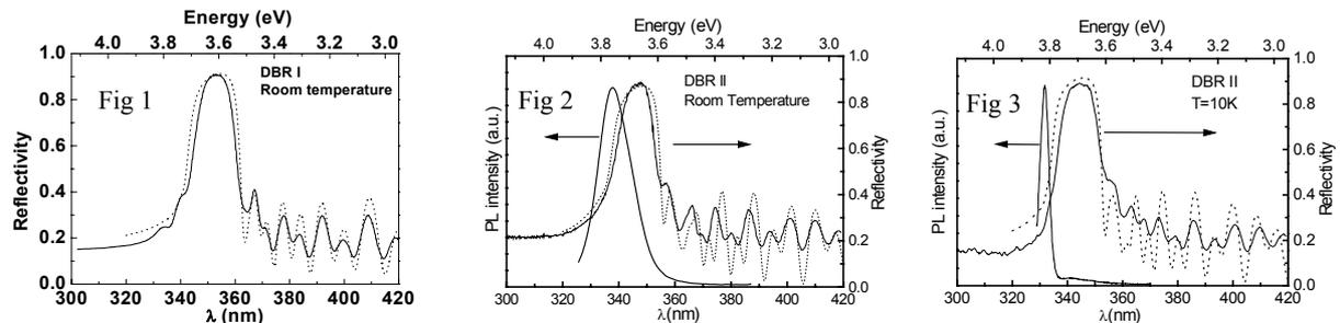
Figs 1, 2 and 3. Reflectivity and PL spectra for DBRs with stop bands peaking at 353nm (Figs 1 and 3) and 347nm. (Fig 2). Full lines experimental, dotted TMR simulations.
