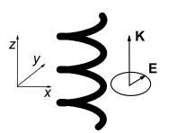
The light absorption by a spiral quantum wire is strongly subjected by the transformation of almost uniform electric field of electromagnetic wave (EMW) to spiral coordinates. In this system the circularpolarized EMW transforms to the running wave with the wavelength determined by the spiral period; the direction of propagation depends on the light polarization and the direction of the spiral. The artificial reduction of wavelength allows the collisionless absorption of light by free electrons.
