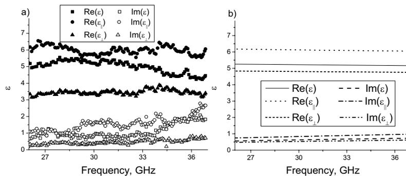
**Figure:** (a) Experimental data of dielectric permittivity of deformed CNT/PMMA composite. (b) Calculated permittivity of deformed CNT/PMMA composite ( $\epsilon$  - permittivity of not deformed composite,  $\epsilon_{\perp} = \epsilon_x = \epsilon_z$ ,  $\epsilon_{\parallel} = \epsilon_y$  – diagonal components of dielectric permittivity tensor of deformed along  $y$ -axis composite).
