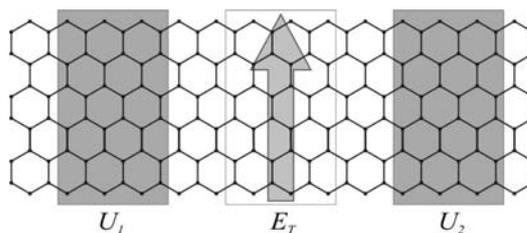
Schematic of a zigzag nanoribbon based quantum pump device. Pumping is achieved by a cyclic variation of gate voltages  $U_1$  and  $U_2$ . The symmetry between up-spins and down-spins is broken by a transverse electric field  $E_T$  (or by a defect – not shown).
