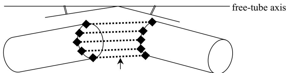
Supercell model of (8,0) tube of 192 atoms is divided on 2 cylinders, whose axes make a fracture. 5 of 3 C–C bonds between undistorted half-tubes are shown by dashed lines.
