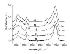
DND spectra of a) initial purified DND b) Z+ c) Z-d) Cu<sup>2+</sup> modified DND e) Co<sup>2+</sup> modified DND.
