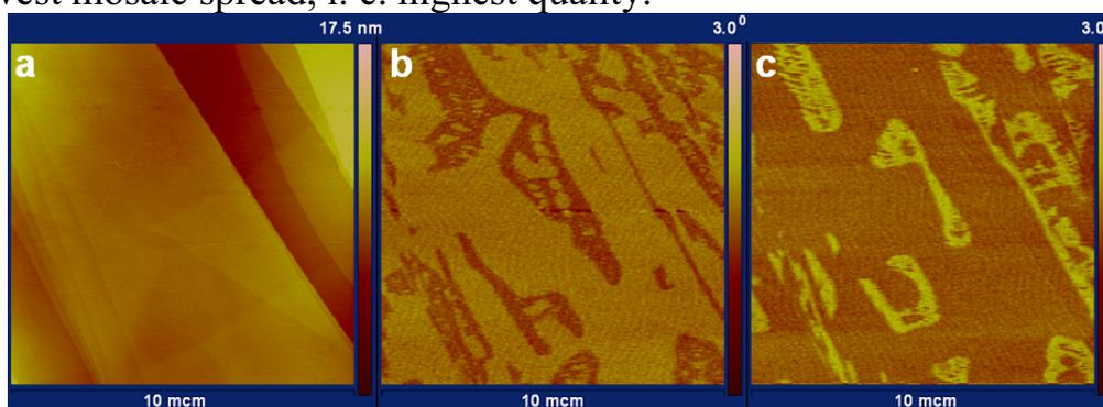
**Figure 1.** EFM images of HOPG graphite: a – topography, b, c – phase images taken at +2V and -2V, respectively.
