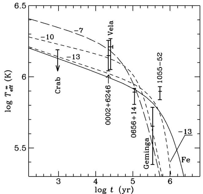
FIG. 2.—Standard cooling of a NS with a nonaccreted envelope, and partially and fully accreted envelopes, compared with observations of thermal radiation from six pulsars (Table 1). The numbers along the curves give  $\log \Delta M/M$ .
