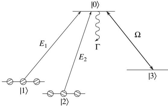
Level scheme of tripod atoms interacting with two weak fields  $E_1, E_2$  and a strong driving field of a Rabi frequency  $\Omega$ .
