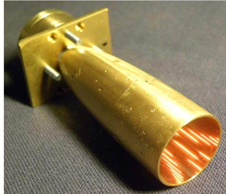
Simulations confirm that about half of the modes collected by the Winston horn actually couple to the bolometer absorber (in single-polarization detectors).
