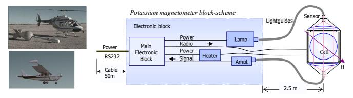
Constructively Potassium magnetometer consists of the sensor the electronic block and the power supply block. The electronic block is connected with the sensor by multi-fiber lightguides and the coaxial cables. Total energy consumption is about 65 W. The electronic block is connected with user's computer and the power supply block with cable up to 50 m length.
