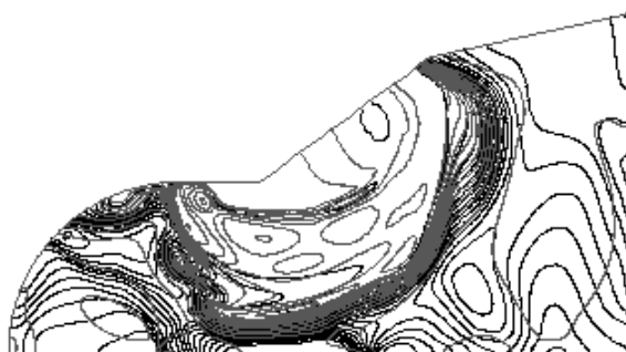
Figure 2. Isopicts (black) and level lines of temperature at the beginning of cycle
