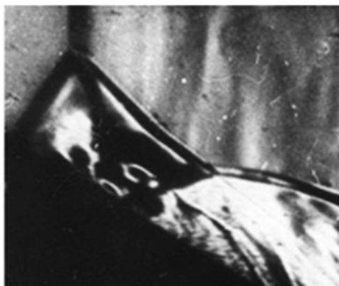
Figure 4. Schlieren picture of shock wave reflection from a wedge in \text{CO}_2 gas, M_0 = 5.18 , \alpha_0 = 32^\circ , p_0 = 20 \text{ torr} .
