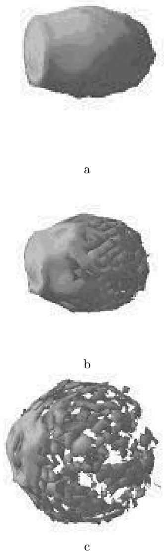
Figure 4. Undermining of ogival shell: a — 30 mcs, b — 50 mcs, c — 100 mcs
