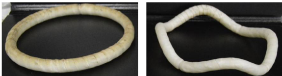
Figure 3. Schematic view of a toroidal ballute, Not deformed ballute (Left), Deformed ballute (Right)
