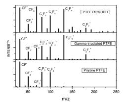
An additional "low temperature" gas release was observed from copolymer FEP (near 500°C) and  $\gamma$ -modified PTFE (near 450°C) as well. And again, as in the case of UDD/PTFE composite, mass spectra indicate the desorption of high molecular fragments absent in pristine PTFE. Notice that both UDD/PTFE and  $\gamma$ -PTFE samples exhibit increased wear resistance compared to pristine PTFE (though it was much higher in the case of  $\gamma$ -PTFE).
