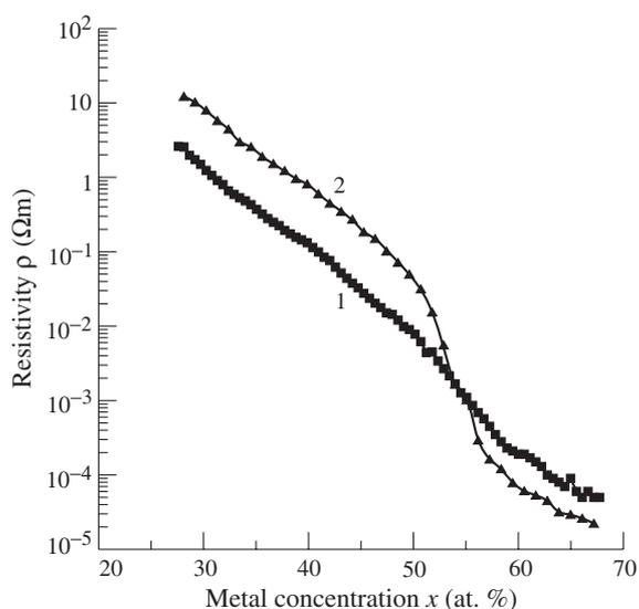
**Figure 5.** Electrical resistivity  $\rho$  of granular structures  $(\text{a-SiO}_2)_{100-x}(\text{Co}_{0.4}\text{Fe}_{0.4}\text{B}_{0.2})_x$  versus the metal concentration  $x$ : 1, as-sputtered; 2, annealed at  $400^\circ\text{C}$ .
