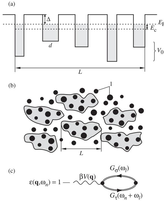
**Figure 8.** (a) Energy structure of a CES. Random distribution of depths  $V_0$  of potential wells in a granule are determined by random variation of granule capacitances.  $L$  is the CES localization size. (b) CES in a granular structure: 1, granules. (c) RPA approximation diagram for the dielectric constant determined by the CES dipole polarization.
