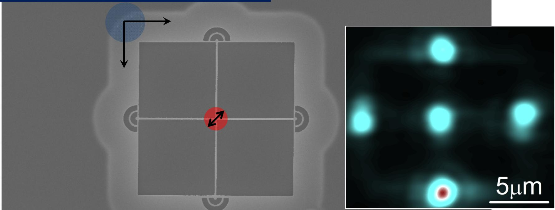
Emission from QDs excited at intersection transmitted along the waveguides and scattered vertically by out-couplers.
